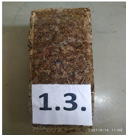
Figure 12. 30 min to sample 1. during exposure to a thermal temperature of 500 0 C
