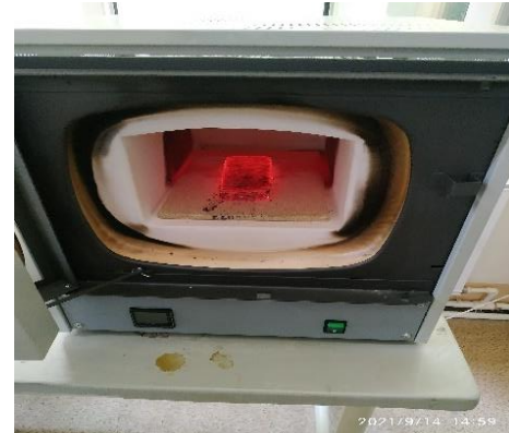
Fig. 14 30 min to sample 3. during exposure to a thermal temperature of 700 0 C
