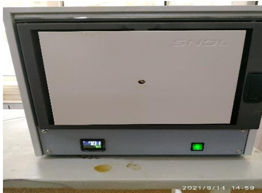
Fig. 14 30 min to sample 3. during exposure to a thermal temperature of 700 0 C
