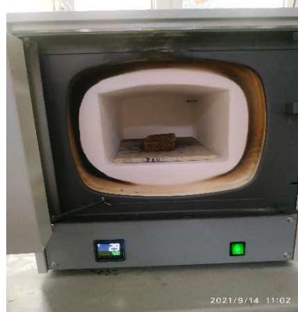
Figure 12. 30 min to sample 1. during exposure to a thermal temperature of 500 0 C
