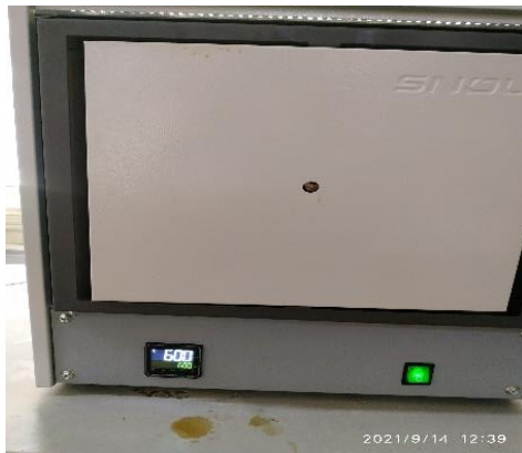
Figure 13 30 min to sample 2. during exposure to a thermal temperature of 600 0 C
