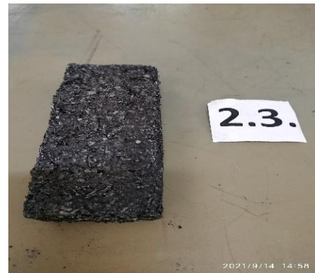
Figure 13 30 min to sample 2. during exposure to a thermal temperature of 600 0 C
