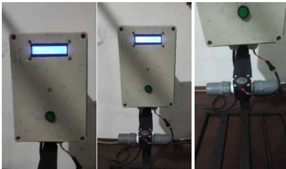
Figure 4. Wastewater Treatment Plant Outlet Water Flow Recording Device
