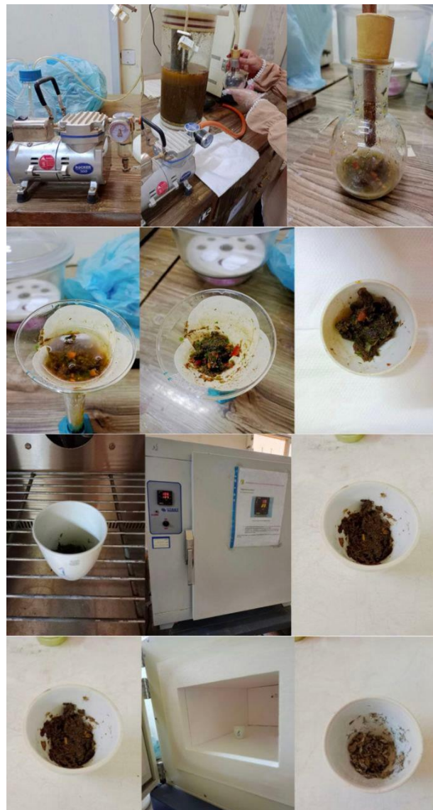
Figure 7: Steps of samples' withdrawal from the anaerobic digester (left to right).
