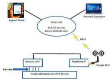
Figure 4. Block diagram of the suggested SCADA model utilized for low cost applications based upon the Arduino LaRo Arduino LoRa Transmitter (ALT) scheme [12].
