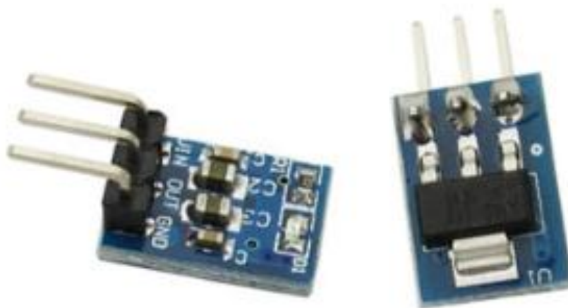
Figure 2. AMS1117 is a 3.3 V power supply module based on the 3.3 V chip.
