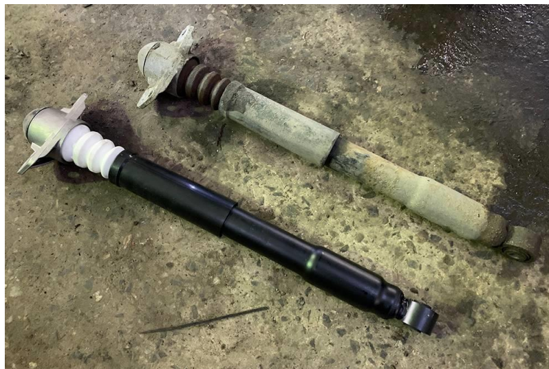
Figure 3. Failure condition of shock absorbers.
