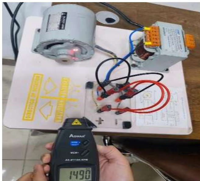
Figure 11. R.P.M. Lazer Digital Tachometer for Measuring Motor Speed
