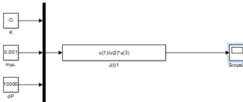
Fig. 1. Block diagram for calculating filtration velocity according to Darcy's law in MATLAB/Simulink
