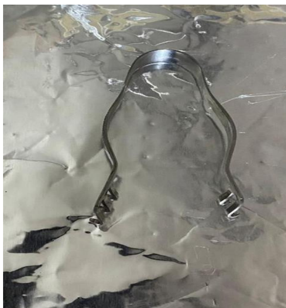
Figure 24 . One of the medical surgical instruments on which the test was conducted, (a hook or retractor instrument called "FINSEN Modified Retractor")
