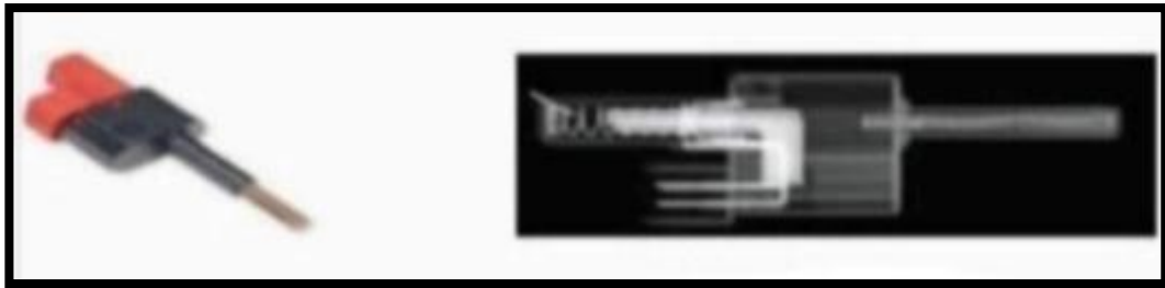
Figure (10-3) Digital X-ray image, components, car key, testing, internal components
