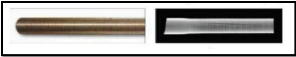
Figure (7-3) Detecting industrial defects or resulting from the use of pipes using X-ray imaging
