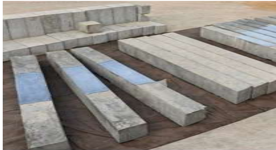
Fig.6: specimen preparation prior to CFRP bonding.
