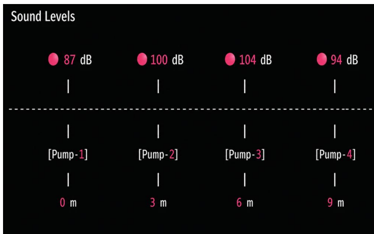
Figure 2. Noise measurement points in the pumping station room
