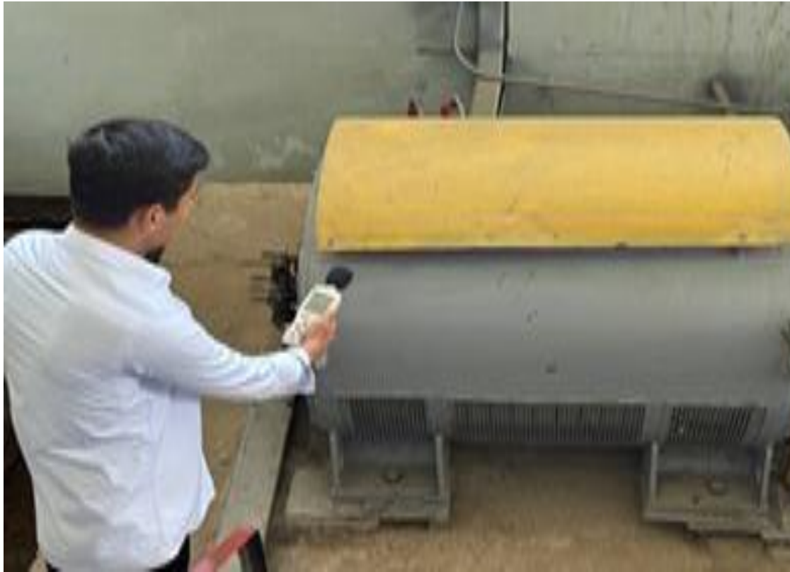
Figure 8: Noise measurement process (ToshGRES pumping station)
