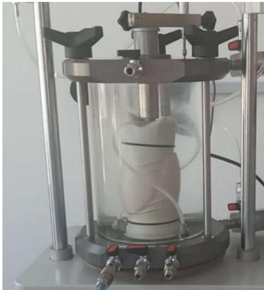
Figure 1. Dune sand specimen in the triaxial cell after failure
